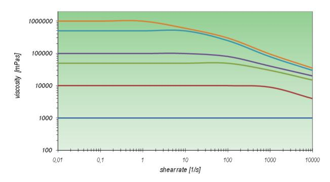
It can be seen in general, that with increasing viscosity of the **KORASILON® Fluid M** the *Newtonian area*, the interval where viscosity is independent from shear rate (indicated by the horizontal part of the curve) is decreasing, while shear thinning behaviour (viscosity is decreasing with increasing shear rate) is becoming more and more evident.
