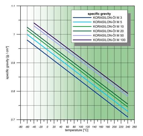
The temperature/specific-density curve of **KORASILON<sup>®</sup> Fluids M 100** is describing the temperature dependency of any **KORASILON<sup>®</sup> Fluids M** with viscosities higher than 100 mm<sup>2</sup>/s.
