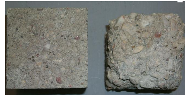
Sample after freeze/thaw-exposure Left with impregnation agent, right without (after approx. 50 cycles)
