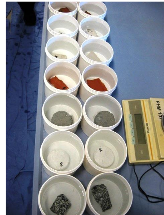
Sample for immersion storage test carried out with different building material
