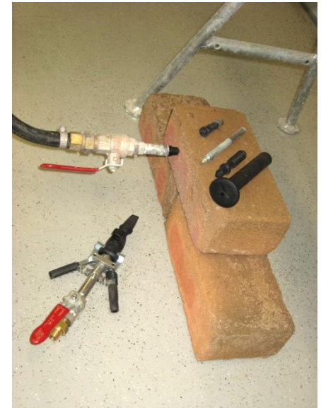
Examples of different packers and injection nozzles as well as different couplings for pressure pumps
